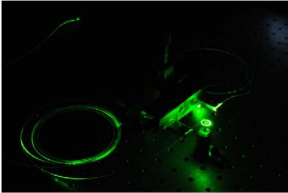
*Millimeter-size whispering-gallery mode resonator coupled with a green laser. The photons, which interact quantum-mechanically, are trapped for about a microsecond inside the cavity and perform around 10000 round-trips before being annihilated.*
